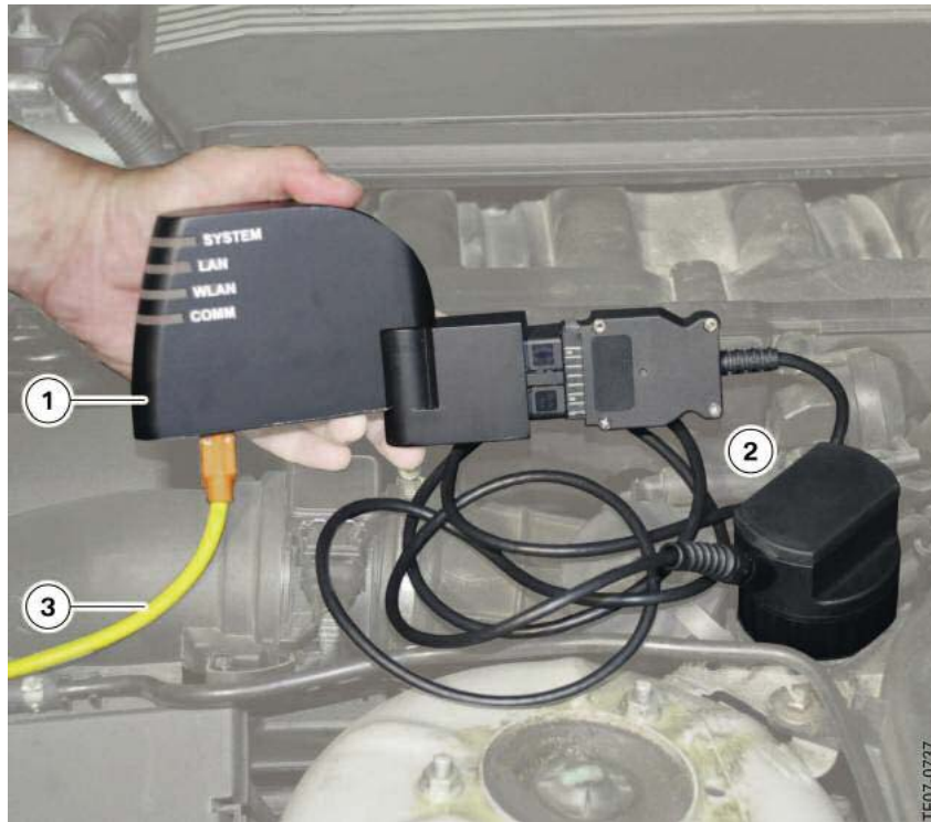
View of the ICOM A and ICOM C connected to a vehicle.
